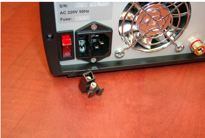
Fig.5. Two fuses in fuse holder including one spare (upper in the figure).
