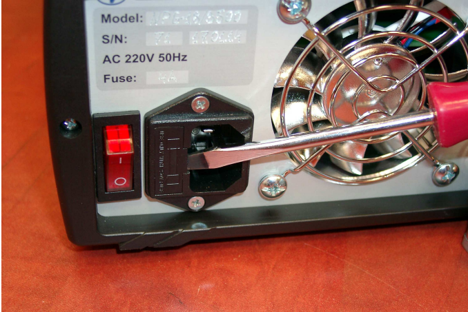
Fig.4. Removing of the fuse holder by flat screwdriver.
