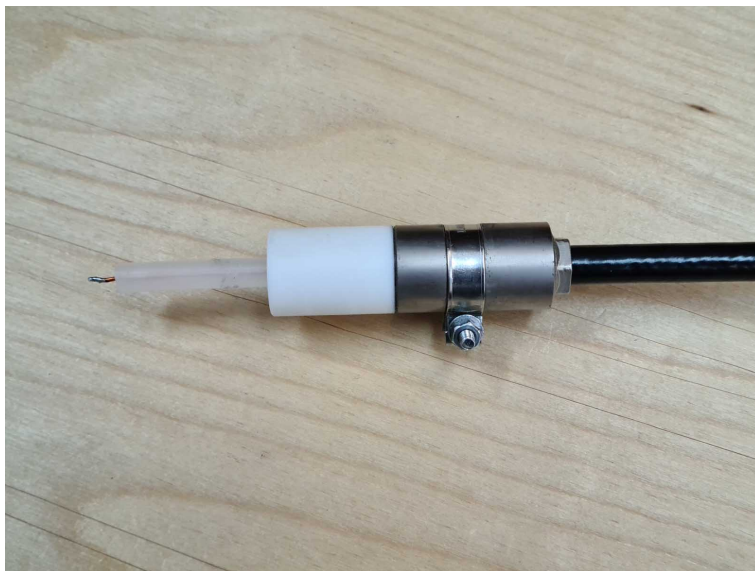
Fig.2. The Teflon cone protection on the load side of the HV coaxial cable.
