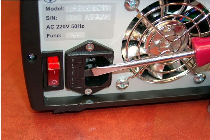
Fig.13. Removing the fuse holder with a flat screwdriver.
