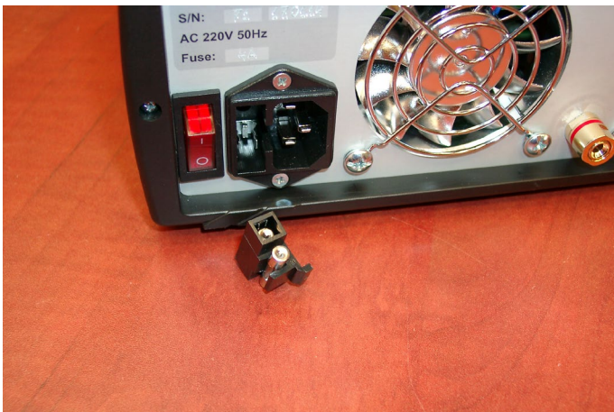
Fig.14. Two fuses in fuse holder including one spare (upper in the figure).
