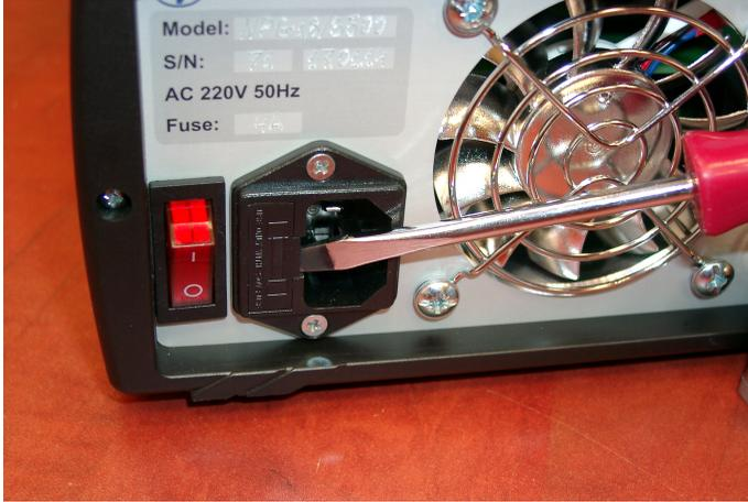
Fig.12. Removing the fuse holder with a flat screwdriver.
