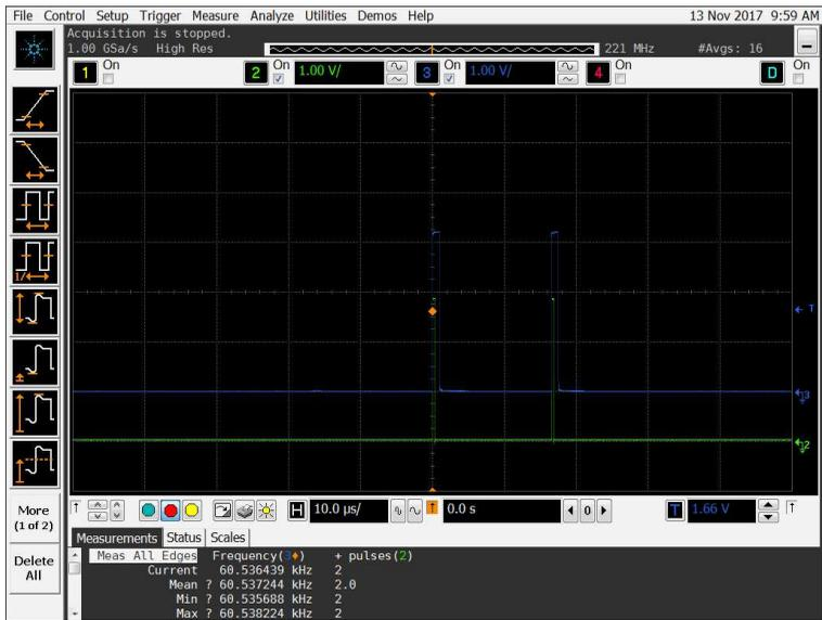
Fig.6. External triggering, burst mode. External triggering pulses (CH3, blue line) set 60 kHz repetition rate and 2 pulses in a burst. CH2 (green line) shows SYNC OUT pulses.
