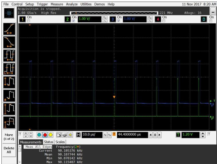
Fig.5. External triggering mode. The external triggering pulses define the repetition rate. CH2 (green line) shows SYNC OUT pulses. CH3 (blue line) shows the triggering pulses fed to SYNC IN connector.
