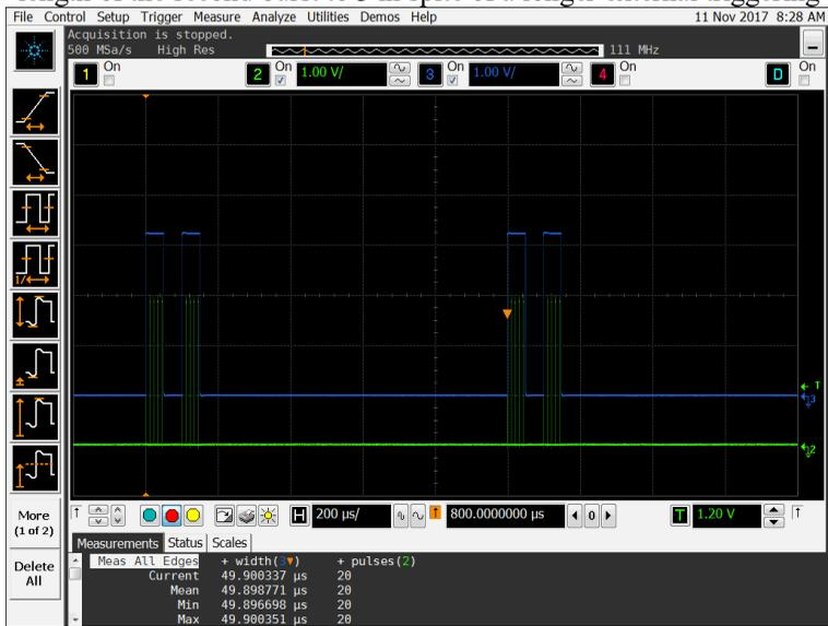
Fig.10. External triggering, burst enable mode. The pairs of SYNC IN pulses (CH3, blue line) set the pair bursts of output pulses (CH2, green line).
