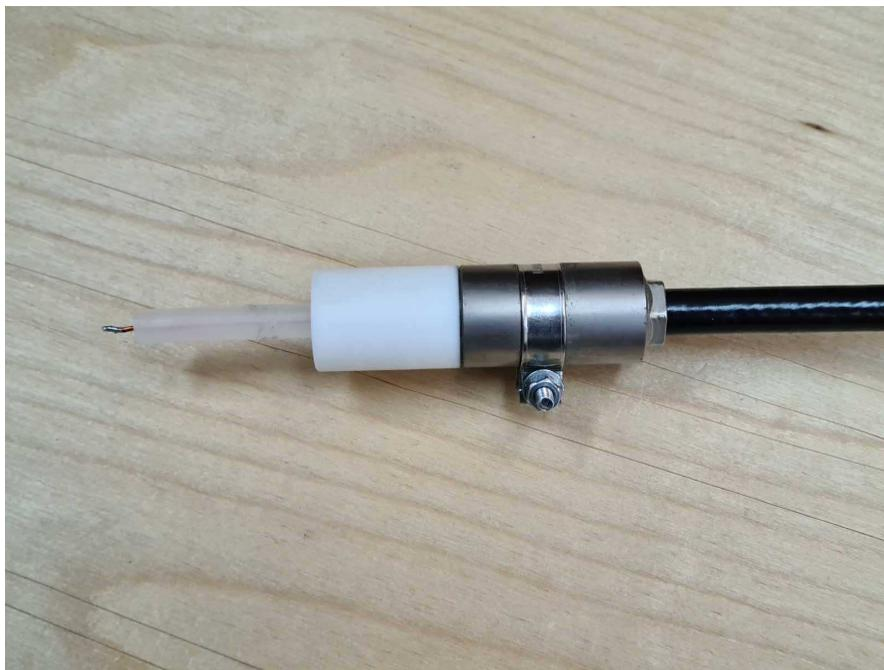
Fig.2. Teflon cone insulator on the cable end.
