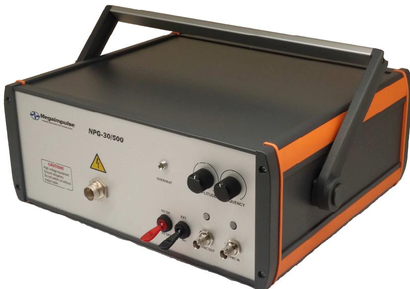
Fig.1. General view of NPG-30/500 nanosecond pulse generator.
