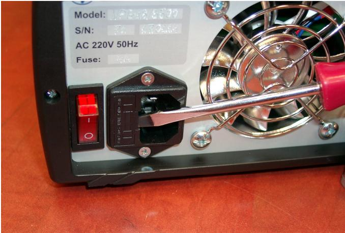
Fig.4. Removing of the fuse holder by a flat screwdriver.
