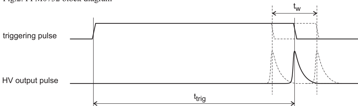
Fig.3. Output HV pulse synchronization with the triggering pulse falling edge
