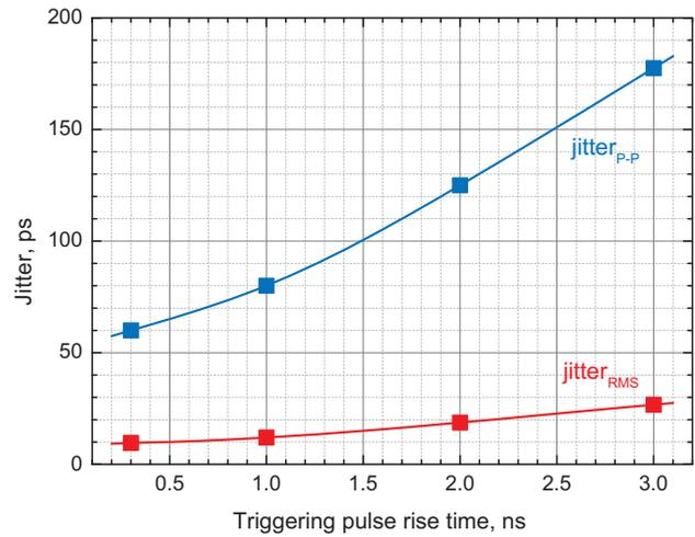
Fig.3. Output pulse jitter<sub>RMS</sub> and jitter<sub>P-P</sub> VS triggering pulse front rise time.
