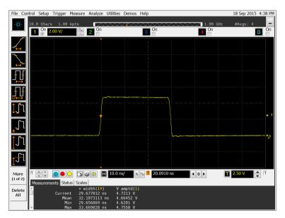
Fig. 3. Recommended triggering pulse waveform.
