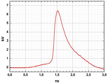
Fig.2. PPM0731 typical output pulse waveform on 50 Ohm matched load.
