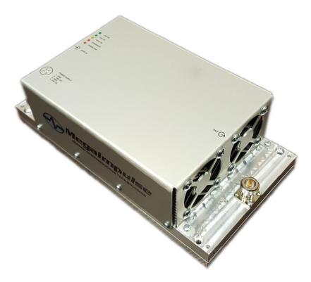
Fig.1. General view of PPM0411 subnanosecond pulse generator module.
