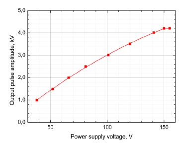
Fig.3. PPM0411 output pulse amplitude VS high voltage power supply.
