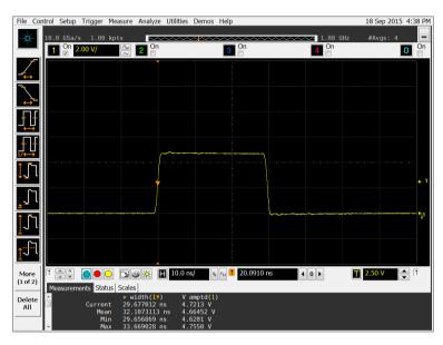
Fig. 4. Recommended triggering pulse waveform.
