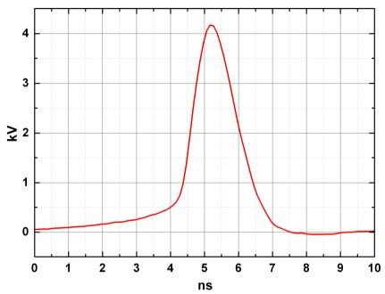
Fig.2. PPM0411 typical output pulse waveform on 50 Ohm matched load.
