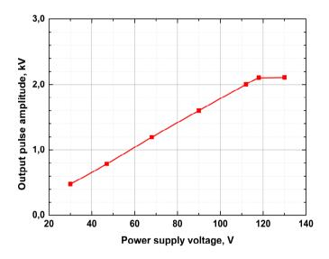
Fig.3. PPM0211 output pulse amplitude VS high voltage power supply.
