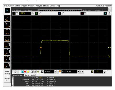
Fig. 4. Recommended triggering pulse waveform.
