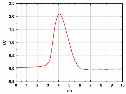
Fig.2. PPM0211 typical output pulse waveform on 50 Ohm matched load.
