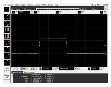
Fig. 3. Recommended triggering pulse waveform.
