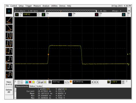
Fig. 3. Recommended triggering pulse waveform.
