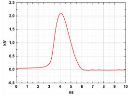
Fig.2. PPG-2/1000 output pulse waveform.
