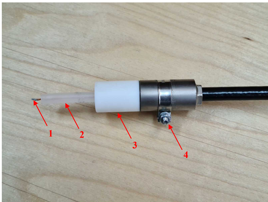
Fig.4. The load side connection: the HV central wire of the coaxial cable (1) in solid PE insulator (2), the Teflon cone insulator (3) which prevents unwanted arcing, and the ground contact (4), i.e. screw and nut on the clamp connected to the coaxial cable braid.
