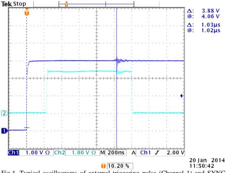
Fig.4. Typical oscillograms of external triggering pulse (Channel 1) and SYNC OUT pulse (Channel 2) of the generator.
