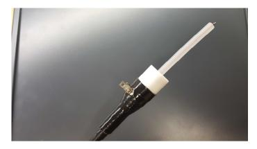
Fig.3. The cone teflon insulator at the cable end.
