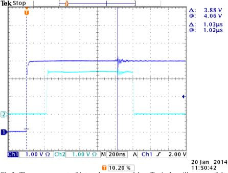
Fig.3. The measurement of internal generator delay. Typical oscillograms of the external triggering pulse (Channel 1) and SYNC OUT pulse (Channel 2) of the generator. The internal delay from the front of the triggering pulse to the high voltage output pulse is about 1  $\mu$ s.
