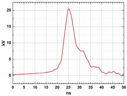
Fig.2. Typical output pulse waveform of NPG-20/3500 on matched 50 Ohm load. Amplitude knob is in max position.
