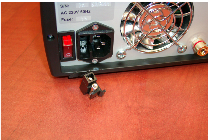
Fig.13. Two fuses in fuse holder including one spare (upper in the figure).
