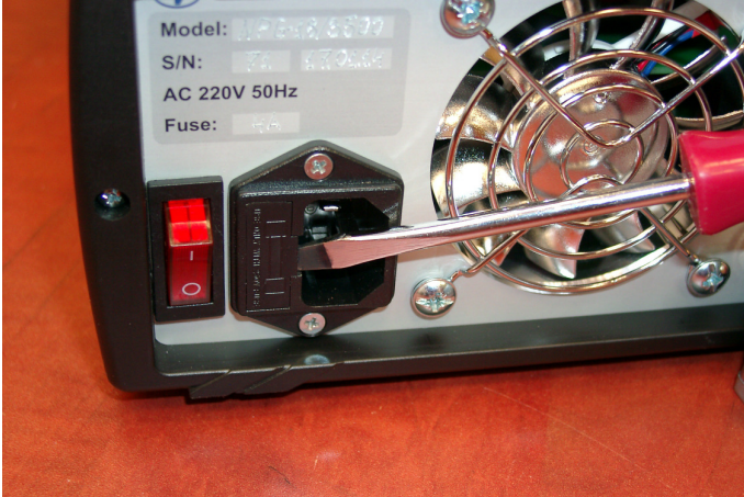
Fig.12. Removing of the fuse holder by flat screwdriver.
