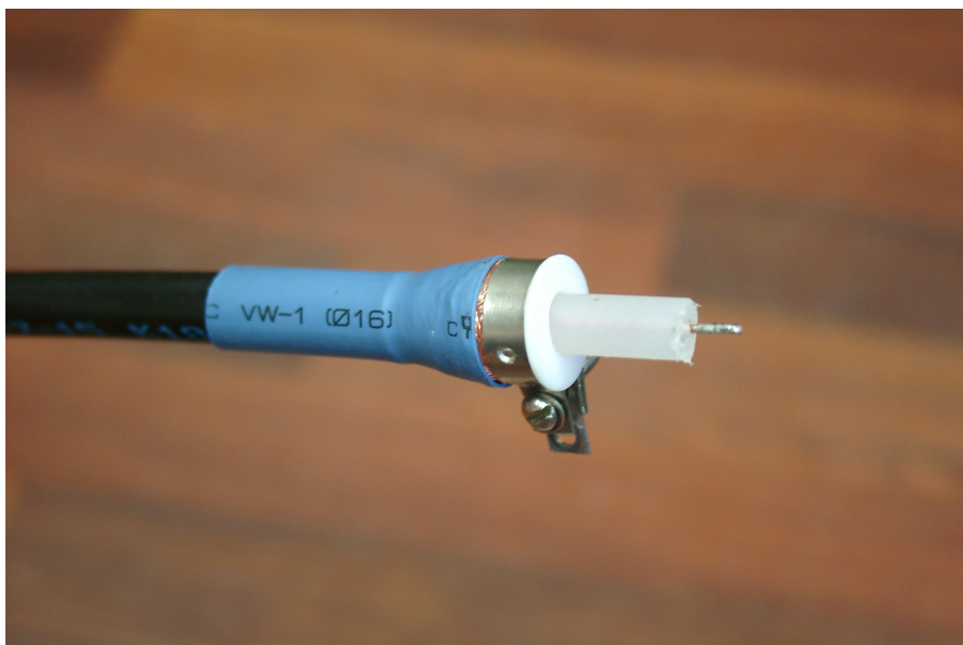
Fig.2. Teflon cone insulator on the cable end.
