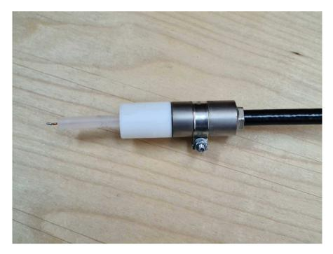
Fig.2. Teflon cone insulator on the cable end.
