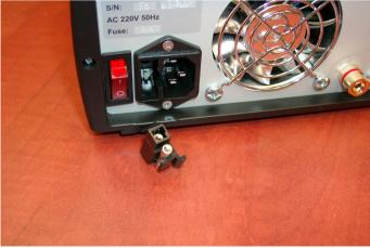
Fig.13. Two fuses in the fuse holder, including one spare (upper in the figure).
