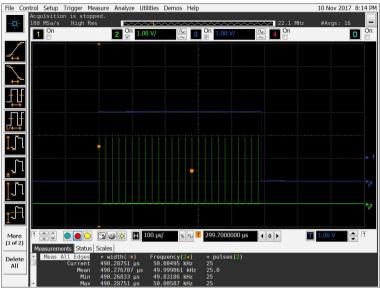
Fig.7. External triggering, burst enable mode. FREQUENCY parameter sets 50 kHz repetition rate within a burst, SYNC IN triggering pulse duration (CH3, blue line) defines the burst length of 25 pulses.
