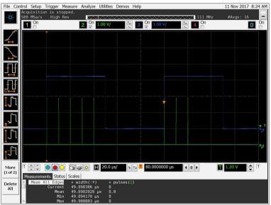
Fig.9. External triggering, burst enable mode. The NUMBER OF PULSES parameter is set to 8, limits the total number of pulses, and reduces the length of the second burst to 3 in spite of a longer external triggering pulse.
