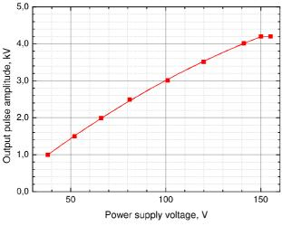
Fig.2. The typical dependence of the output pulse amplitude from high voltage DC power supply.
