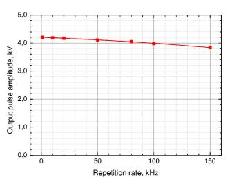
Fig.3. The typical dependence of the output pulse amplitude from repetition rate.
