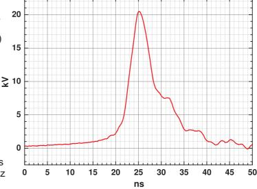
Typical pulse waveform on matched 50 Ohm load
